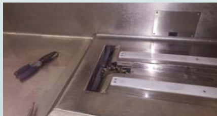
ADDING NEW DRIVE, WEAR STRIPS, BED & COG
