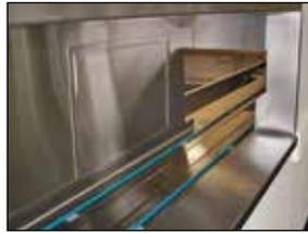
**Slat Belt System** – Caddy's unique slat belt system incorporates thermoplastic resin snap-connect slats. Our unique monorail system travels above the soiled bed and drip tray, providing increased sanitation and ensuring years of trouble-free operation.
