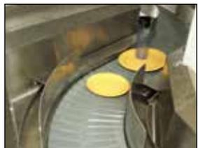
**Caddy Star System** – Built on a heavy-duty 3/16" or 1/4" angle frame with tray towers manufactured of fully welded stainless rod – available with an optional anti-jam tray positioning beam. Tray racks are removable for cleaning. Cantilever design (over the scrapping table) allows a smaller footprint and reduces labor.
