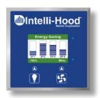
system for commercial kitchen exhaust hoods. Its processor controls the speed of the exhaust and make-up air fans through variable frequency drives (VFDs) based on input signals from temperature probes
